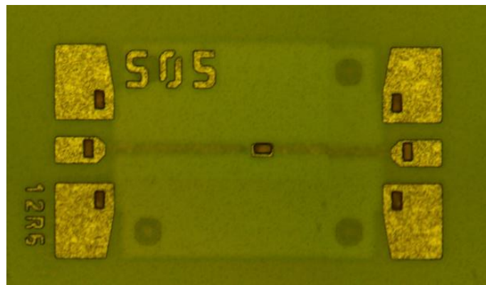
Figure 21: Microscopic image of fabricated test transistor with 0.5 \mu\text{m} emitter width.
