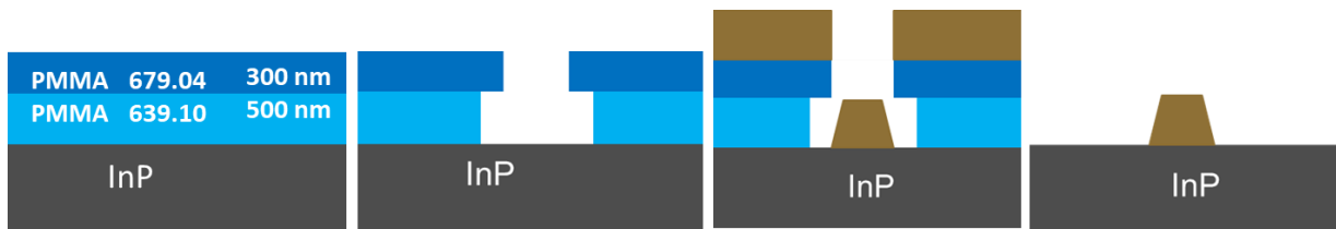
Figure 18: Schematic cross-section of the fabrication of emitter or collector metal layer.
