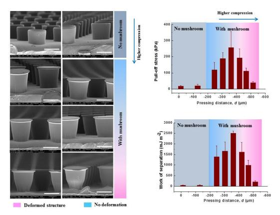
**Figure 1.** Scanning electron micrographs of UA16 micropillars fabricated with different compression (left). Scale bars are 40  $\mu$ m. The dependence of pull-off stress and work of separation on compression (right).
