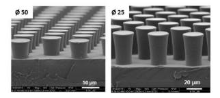
Figure 2. Scanning electron micrographs of the microstructures with pillar diameter of 50  $\mu m$  and 25  $\mu m.$
